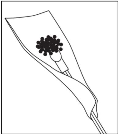
Form a "spoon" of masking tape around the head of an electric match type ignitor. Two ignitors may be used for some redundancy. Place a small amount of ffff black powder or a fine grain black powder substitute, such as Pyrodex, in a pile on the head of the ignitor.
