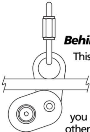
This method requires a small amount of structural modification. Cut a slot about one inch long by one-eighth inch wide in a bulkhead where you have access to the other side. A word of
