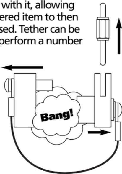
*With the retention bolt removed, the quick link can now slide free.*
