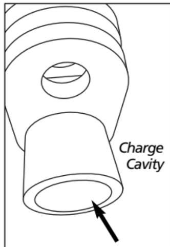
ignitor leads first, into the charge cavity and feed the ignitor leads out the hole in the back of the Tether cup. Pull through until the charge is nearly completely in the cavity
