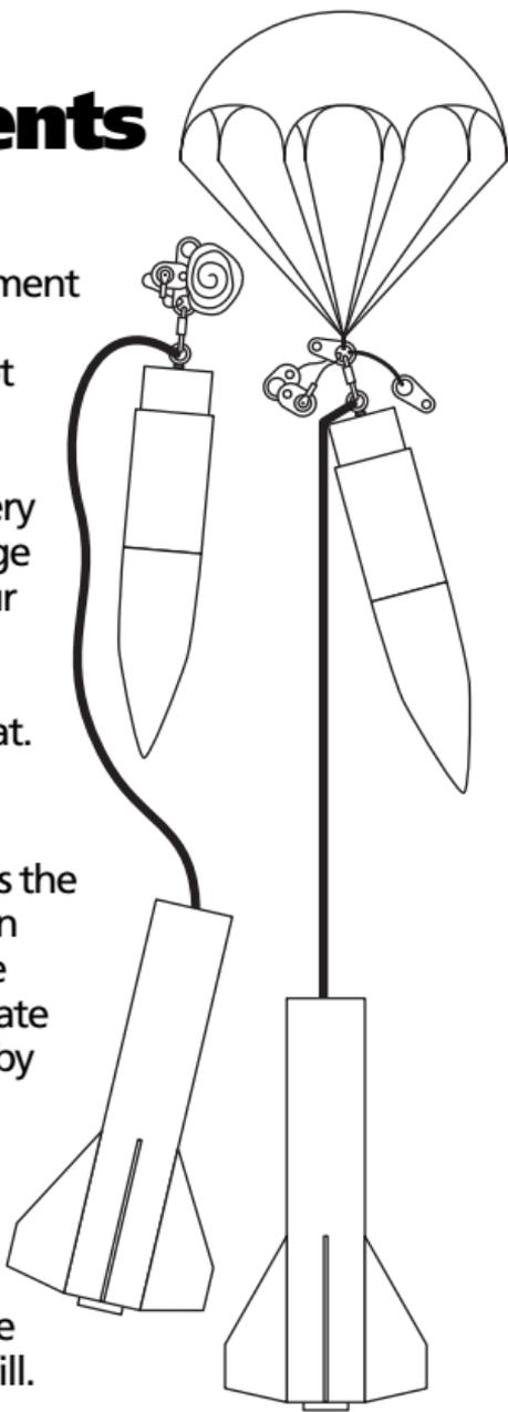
Minimum diameter enthusiasts and smaller rocket flyers will find this useful. Configurations used in this recovery arrangement are *Behind the Mount*, *Behind a Link*, or *In-Line Methods*
