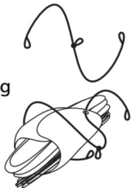
When Tether is triggered, it will release the two loops, the leash will unbind the chute and the main will fall out of the nomex and fill.
