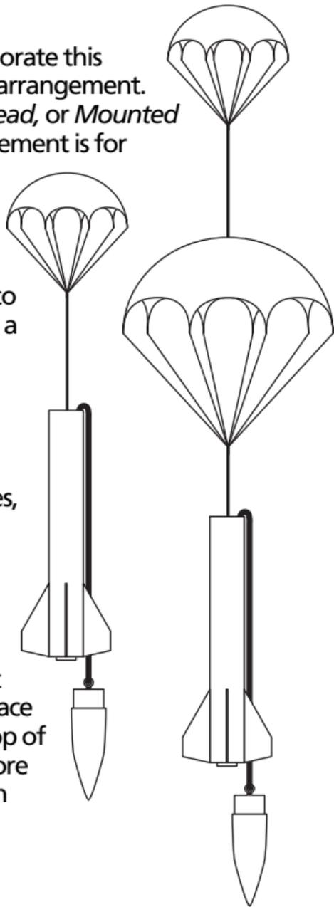
At apogee, the charge inside the wadding will separate the rocket and deploy the drogue chute. The chute will open and pull against Tether. At main deployment altitude, the main event charge in Tether fires, releasing the loop in the line from the drogue to the main, thus allowing the drogue to pull the main out, and the main fills.
